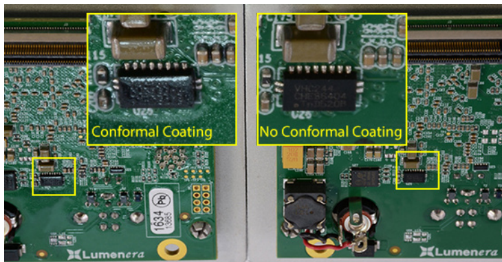
Figure 5.1: Conformal coating versus no conformal coating
