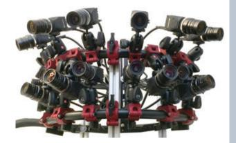
The left image shows the camera array Disney Research constructed for capturing the panoramic videos.
