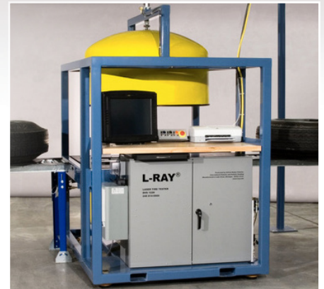
L-Ray Differometric Digital Tire Test Machine Featuring Lumenera CCD Camera
