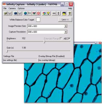
Additionally, a USB 2.0 plug-and-play interface removes the need for framegrabbers and allows fast video. Included is a TWAIN interface, allowing the camera to be used with 3rd party software applications.
