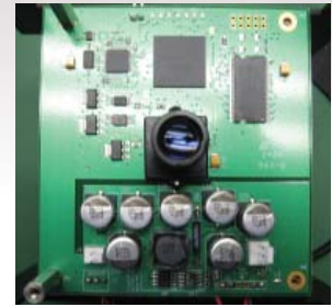
Lumenera’s Lu171M single board camera was customized to meet the customers application needs.
