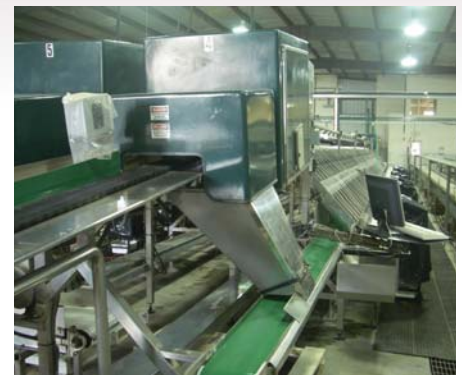
ORAKA's electronic asparagus grader and sorter featuring Lumenera LU075 camera
